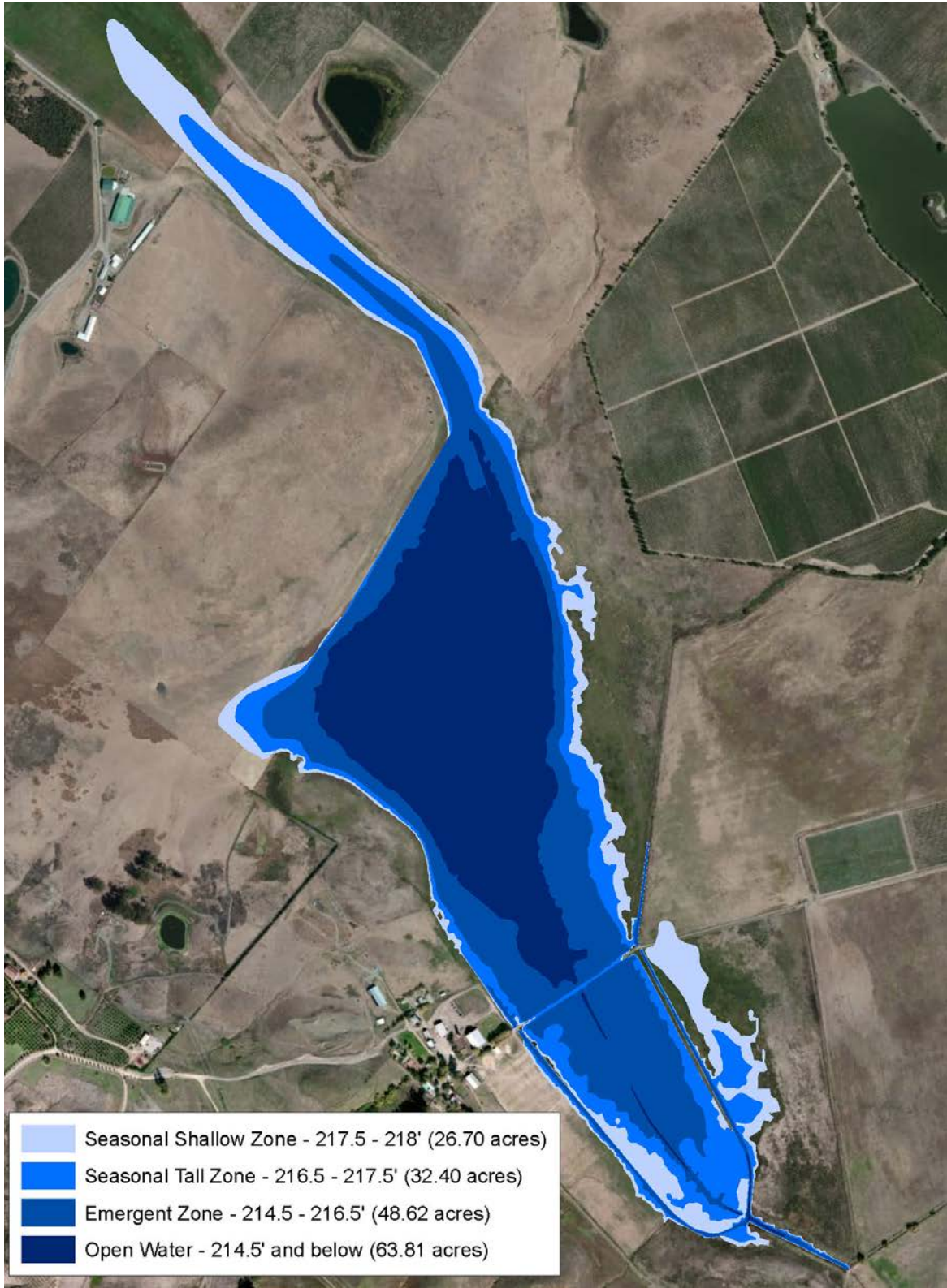
Figure 12. Areas of Inundation for Target Habitats for Restoration Alternative 2 – Lake Outlet Elevation at 218' without a Back-berm.
