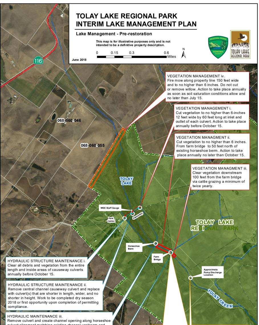
culvert alignment matching existing channel upstream and
